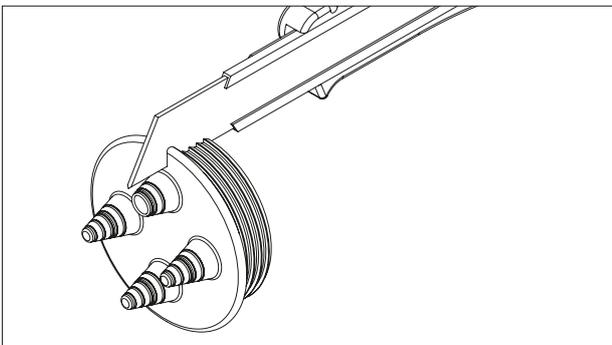
Now press the cable gland into the corresponding sleeve/branch of your vent pipe.
