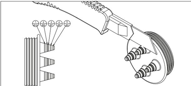
Cut off the nipples accordingly so that you can pull the pump connection cable or the pneumatic hose tightly through the resulting opening.
